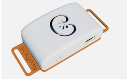
Figure 1: A smart patch for Dialysis patients monitoring that includes a lightweight AI model with the ESP32 MCU using TF lite
